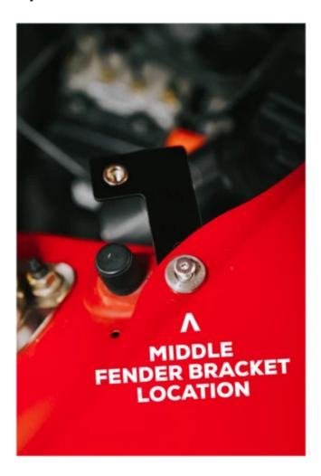
5. Locate this frame rail hole. This will be the location for the frame rail bracket. Install the bracket in the orientation as pictured.
