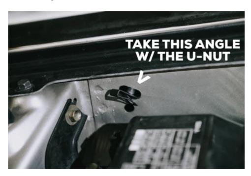
10. Test fit the Allen screw to ensure this bolt can be threaded through. This will help confirm proper alignment.
