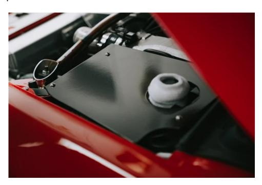
7. We move on to the passenger side battery cover panel. You will reuse the 10MM OEM bolt that is holding in the washer fluid bottle. Remove the bolt and install the single hardware bracket here. Leave slightly loose for final adjustment.
