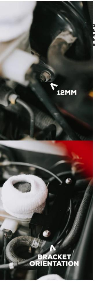
3. Slide in the master cylinder bracket, then finger tighten both nuts allowing for height adjustment. The orientation is as pictured. 4. Remove the middle fender bolt. Slide in the middle fender bracket as pictured. Reinstall the OEM bolt to hold the bracket in place. Finger tighten to allow for final adjustments.
